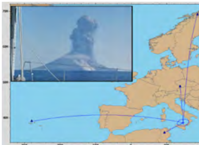
The eruption of the Stromboli volcano, Italy, on 3 July 2019 was used as a training exercise for the intermediate infrasound training held in Bucharest, Romania from 15 to 19 July 2019. The figure displays the obtained eruption location from IMS infrasound observations and visual observation of the eruption (Source: © Y. Xu & S. Berziga / Licet Studios).
