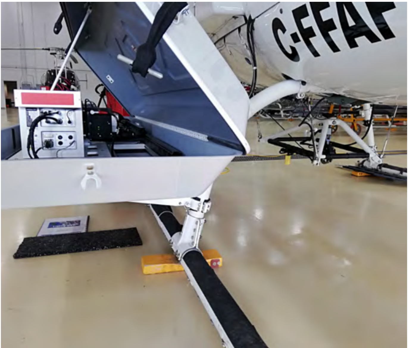
MSIR configuration on an AS350 helicopter during the 2019 OSI third training cycle advanced course on airborne techniques in Canada.
