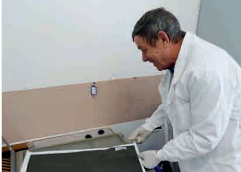
Radionuclide station RN58: filter removed from the air sampler before being compressed.
