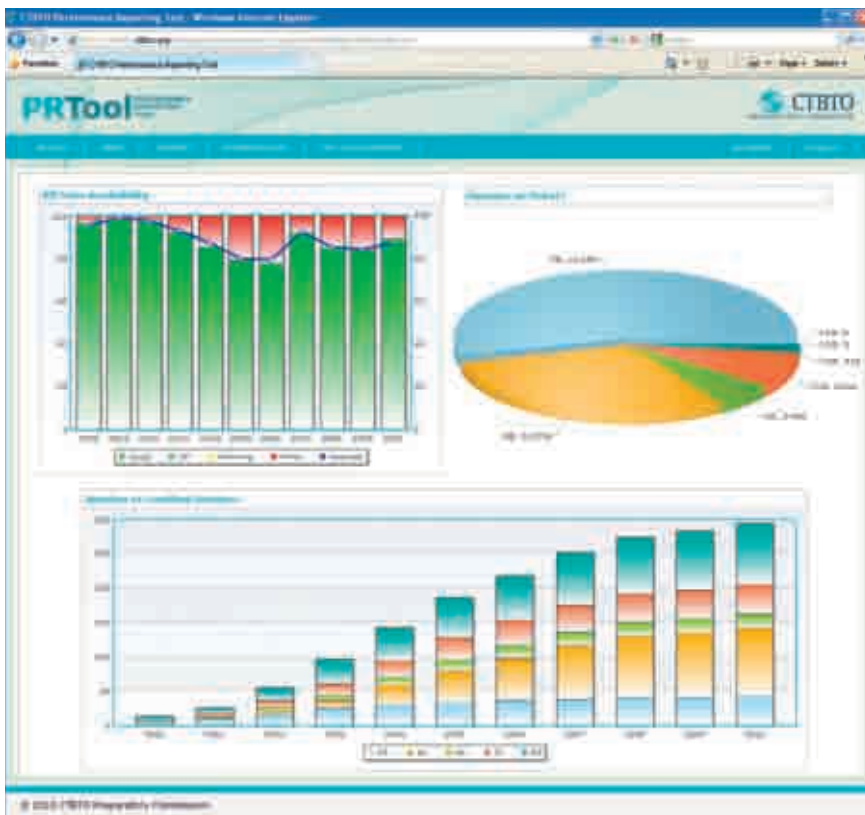
Sample screenshot of verification system metrics displayed by the Performance Reporting Tool (PRTTool). Top left: evolution of data availability of IMS radionuclide stations from 2000 to 2010. Top right: distribution of reports, requests and notifications, by type, received in IDC operations from all IMS facilities in 2010. Bottom: cumulative numbers of certified IMS stations, by technology, from 2000 to 2010.
