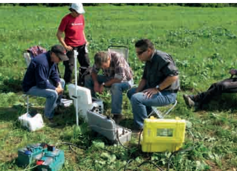
Deep ranging electromagnetic sounding equipment being operated during a field test in Pecs, Hungary, September 2010. Such equipment can be used in the continuation period of an OSI for detection of anomalies caused by artificial structures and the geological equivalents of signals typical of underground nuclear explosions.
