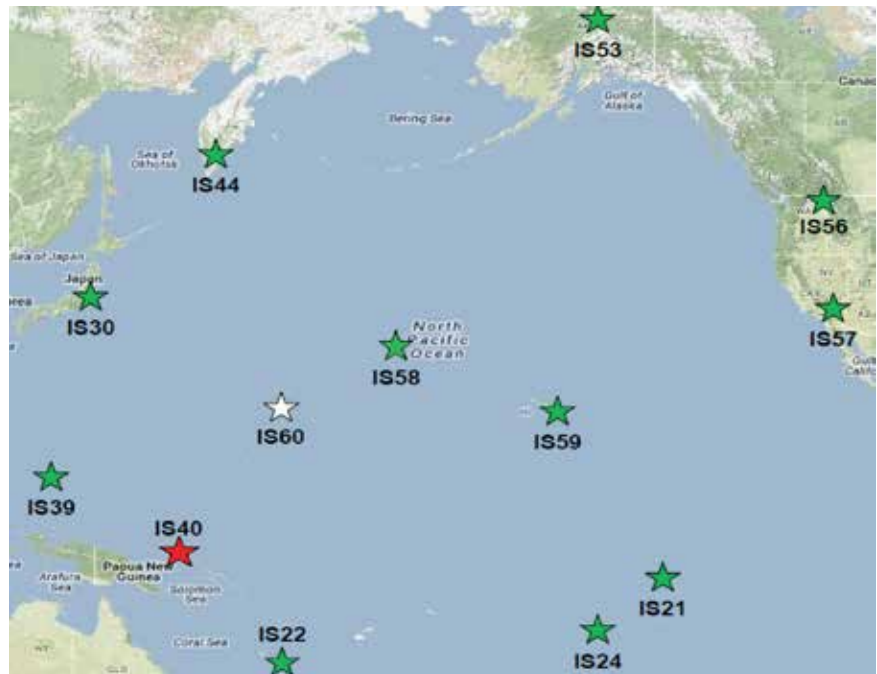
Pacific Ocean IMS infrasound stations around IS40 (red star). Green and white stars respectively represent certified and non-certified IMS infrasound stations.
