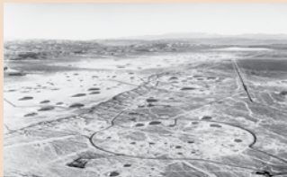
Saucer-shaped craters caused by subsidence following the underground nuclear tests at the Nevada Test Site. Courtesy of U.S. Department of Energy.
