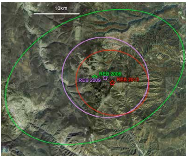
The seismic data registered by the CTBTO's monitoring stations help define the area to be searched under an on-site inspection (OSI). This area has been set at a maximum of 1000 km 2 . The ellipses on the map show the location estimates of the 2006 (green), 2009 (purple) and 2013 (red) declared nuclear tests by North Korea. The CTBTO located the 12 February event to within an area of 181km 2 . (red ellipses). Once the CTBT has entered into force, an OSI can be carried out to search on site for any evidence of a nuclear explosion.
