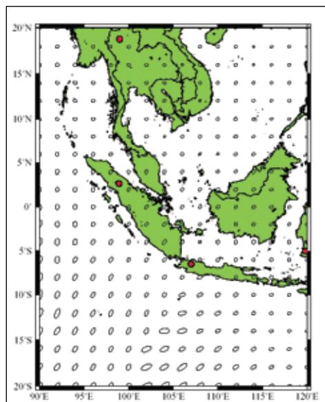
FIG. 3 HORIZONTAL ERRORS OF ESTIMATING EARTHQUAKE LOCATION USING IMS DATA (RED CIRCLES) IN ADDITION TO LISS AND IRIS DATA.
