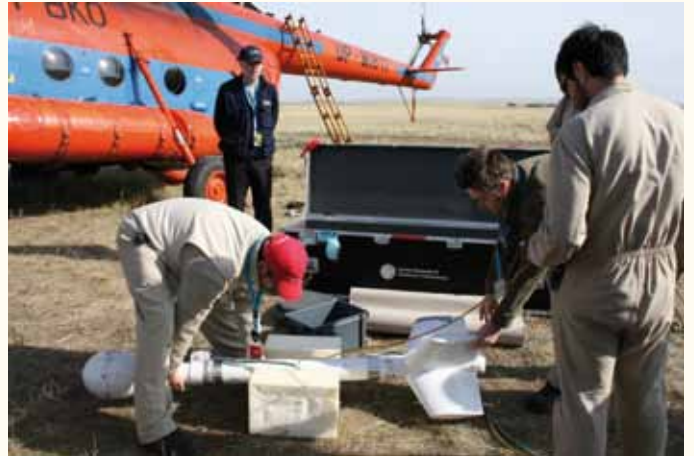
GEOPHYSICISTS PREPARE FOR AIR-BORNE MAGNETIC FIELD MEASUREMENTS.
