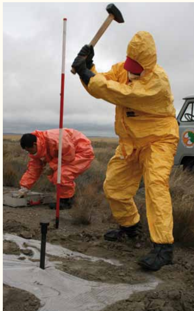
THE TEAM SAMPLED AIR IN THE GROUND TO LOOK FOR THE NOBLE GAS ARGON.
