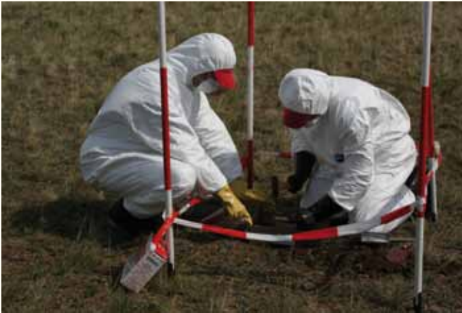
INSPECTORS COLLECT SOIL SAMPLES FOR RADIATION ANALYSIS.
