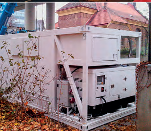
To facilitate measurement of the global radio-xenon background, portable equipment can be deployed temporarily at various sites. Top: Transportable xenon laboratory developed at the Pacific Northwest National Laboratory (USA) using a SAUNA system (Sweden) (host institution: National Nuclear Energy Agency (BATAN), Jakarta, Indonesia). Bottom: Mobile SPALAX system (France) (host institution: Kuwait Institute for Scientific Research, Kuwait City).
