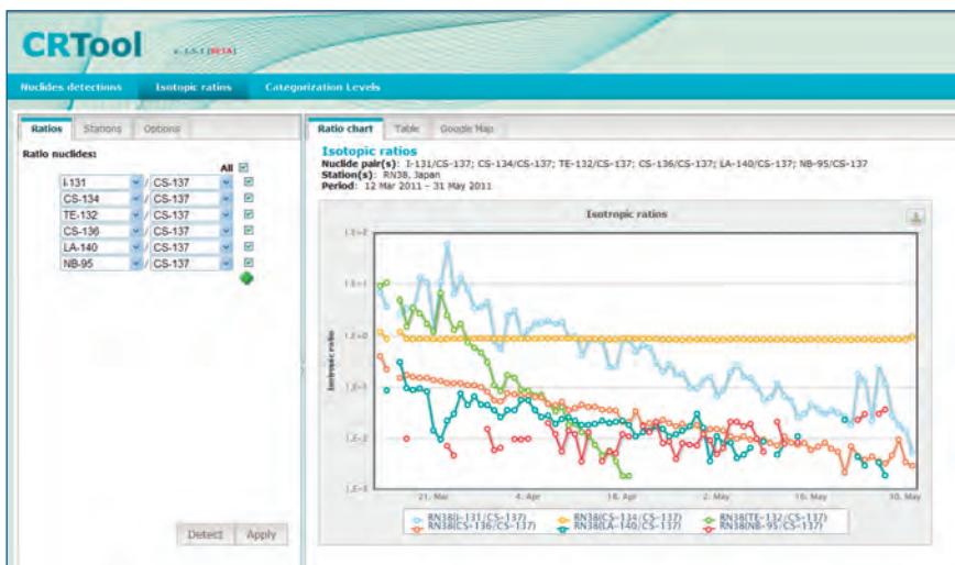
Top: Screenshot of the display produced by PRTool of the monthly average mission capable data availability for all waveform stations in operation. Bottom: Screenshot of the display produced by the concentration reporting tool (CRTool) of the evolution of the activity concentrations of several nuclides recorded at radionuclide station RN38 (Takasaki, Gunma, Japan) after the Fukushima accident.
