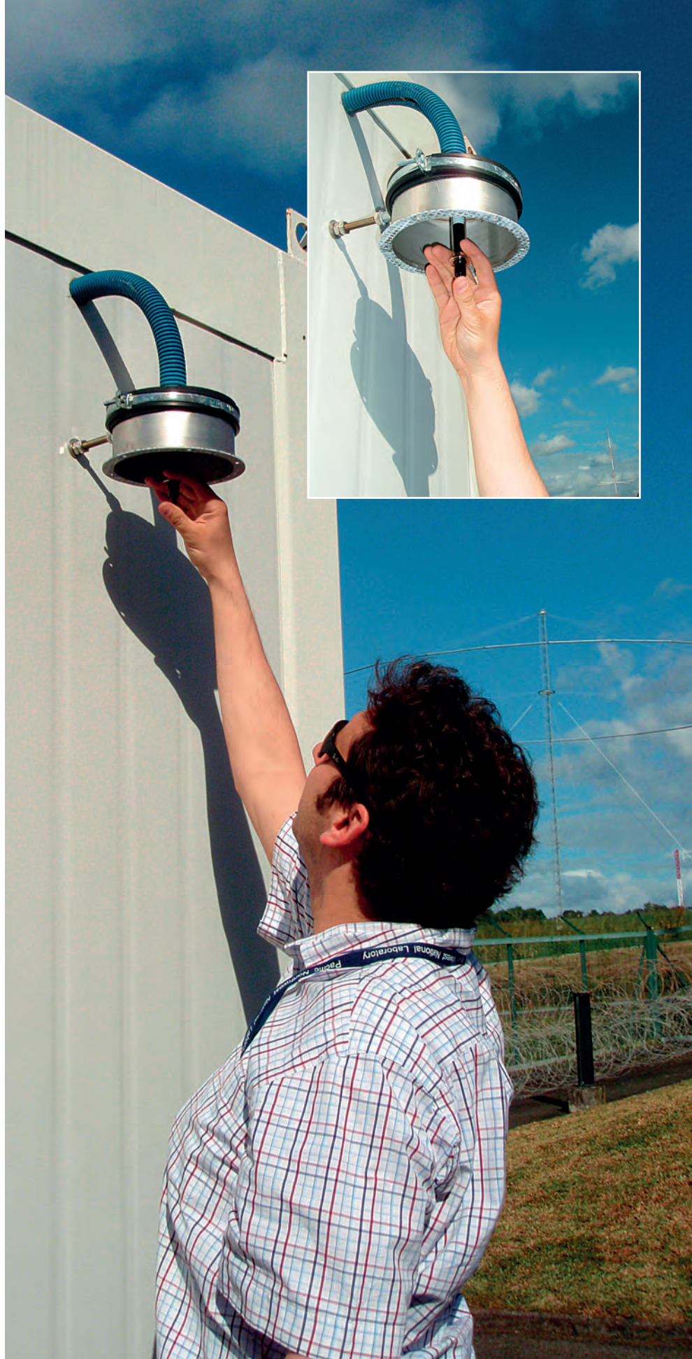
PTS officer performing a spike test during a certification visit to RN29, Réunion (France), in which radionuclides were injected into the monitoring system to assess its performance.
