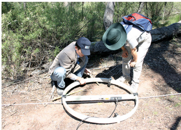
OSI equipment demonstration, Australia: levelling a receiver coil used for measuring induced magnetic fields.
