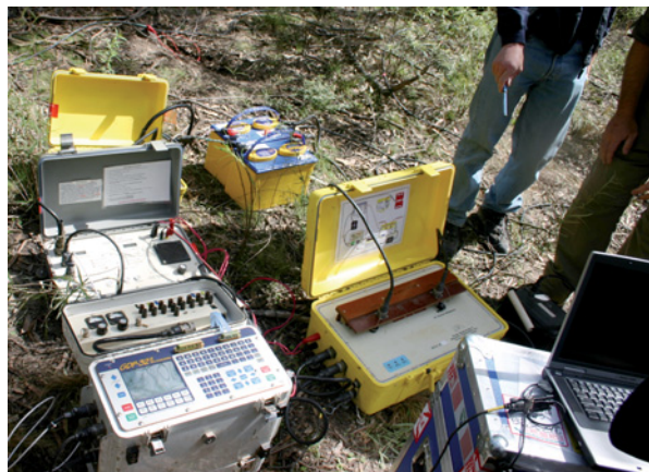
OSI equipment demonstration, Australia: equipment for resistivity measurement.
