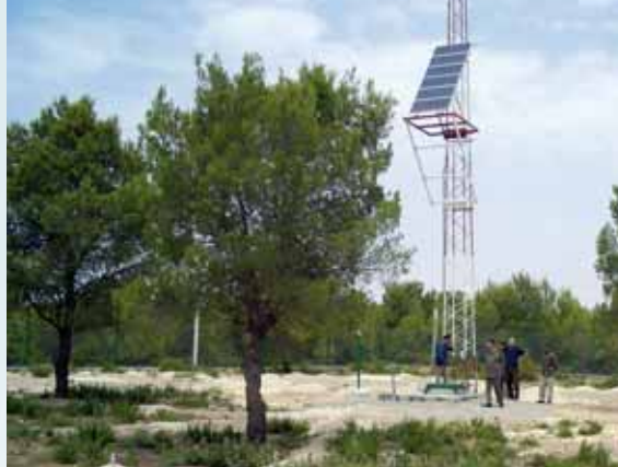
Right: Antenna for infrasound station IS48, Kesra, Tunisia.
