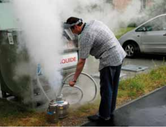
Above: Filling a dewar with liquid argon for cooling the ARIX-3F system.
