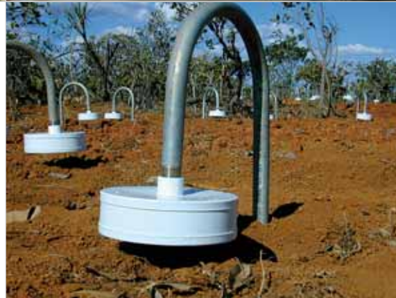
Detail of an inlet port of the wind noise reducing system at infrasound station IS7, Warramunga, Northern Territory, Australia.
