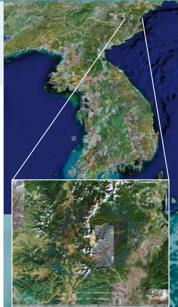
Locations and confidence ellipses for the event of 9 October 2006 in the Democratic People's Republic of Korea. The blue ellipse associated with the location resulting from automatic data processing (and provided in Standard Event List 1) had an area of 2389 square kilometres. In contrast, the red ellipse for the location resulting from the subsequent review by IDC analysts (and given in the Reviewed Event Bulletin) had an area of 880 square kilometres, which is less than the maximum area of 1000 square kilometres allowed for an OSI under the Treaty.
