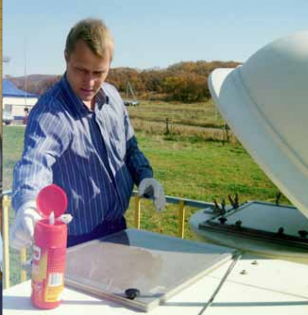
Station operator Andrey Berejnoj changing the filter at radionuclide station RN58, near Ussuriysk.
