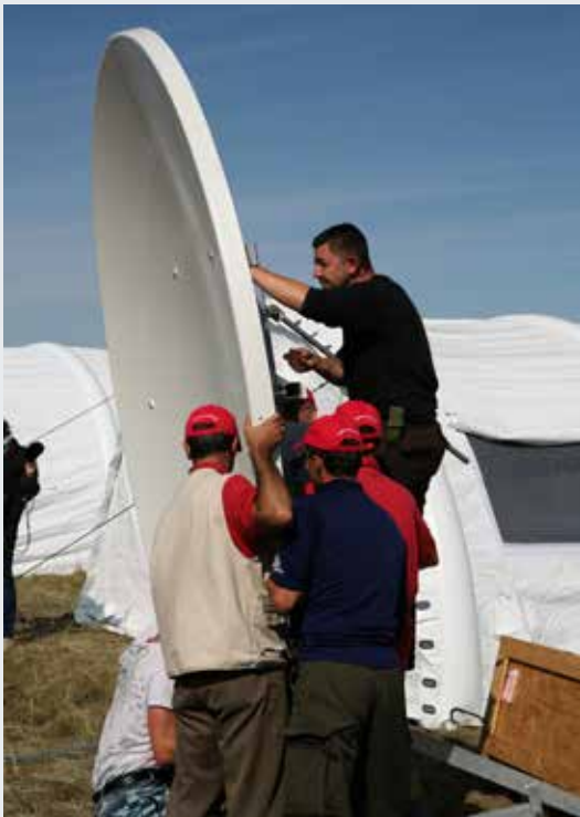
VSAT antenna used for IFE08 (2.4 metres, heavy, six hours to install)
