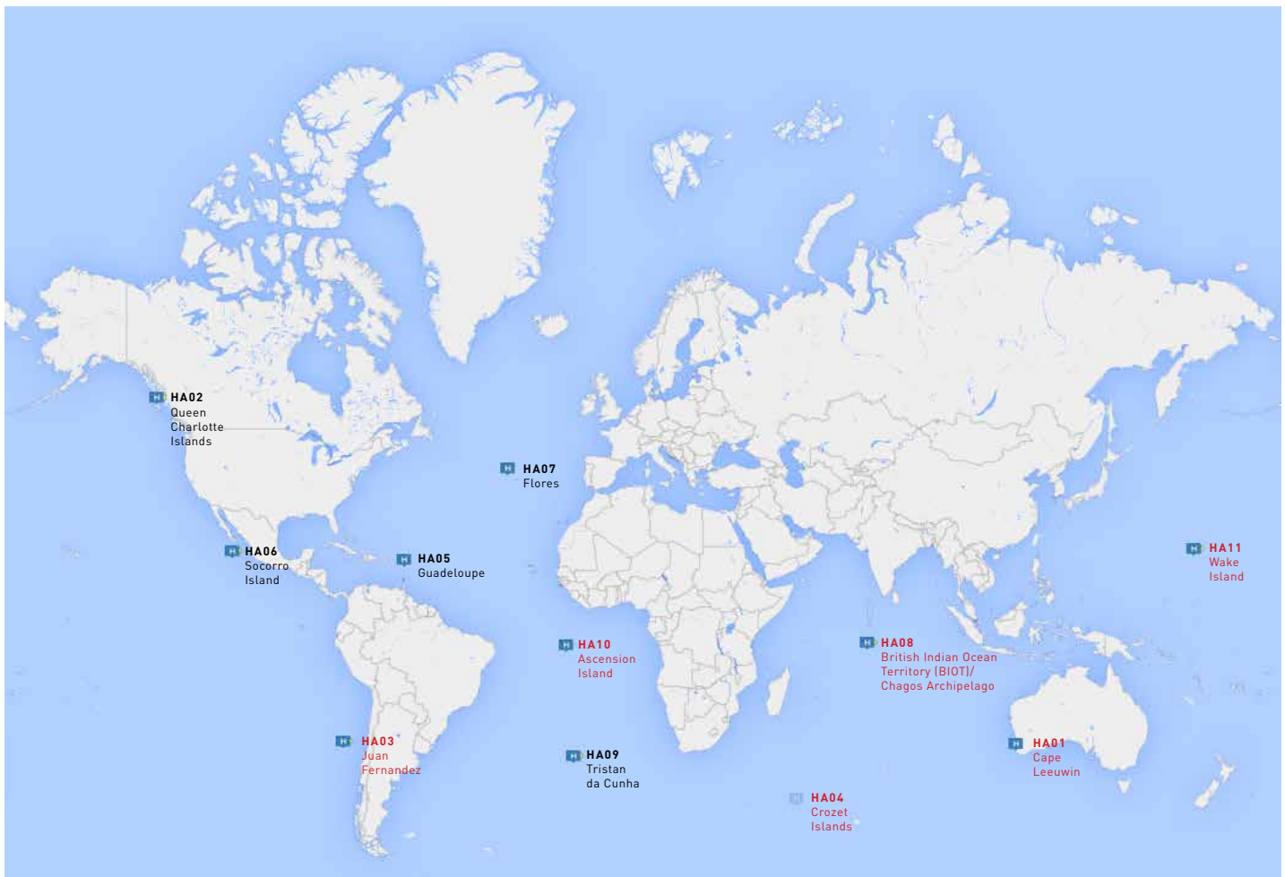
Figure 2. The CTBTO's network of 11 hydroacoustic stations. Stations in red are the hydrophone cabled stations and those in black are the T-phase stations.
