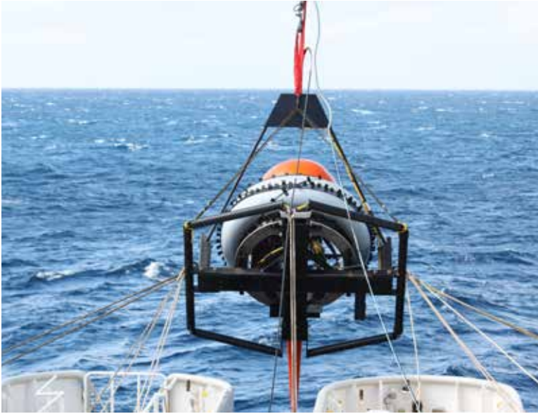
Deployment of a hydrophone mooring in rough seas.
