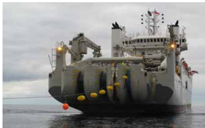
The installation vessel was a modern sub-sea telecommunications cable ship.
