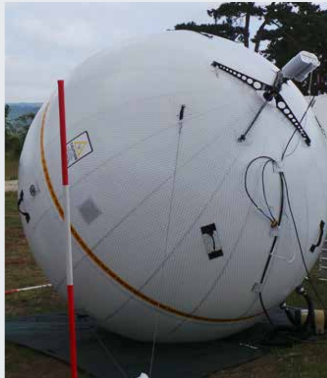
VSAT antenna to be used during IFE14 (30 minutes to deploy, light, field VSAT antenna)
