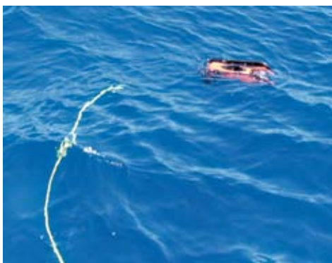
UNDERWATER ROBOT WITH 'UMBILICAL' CABLE, READY FOR INSPECTION DIVE
