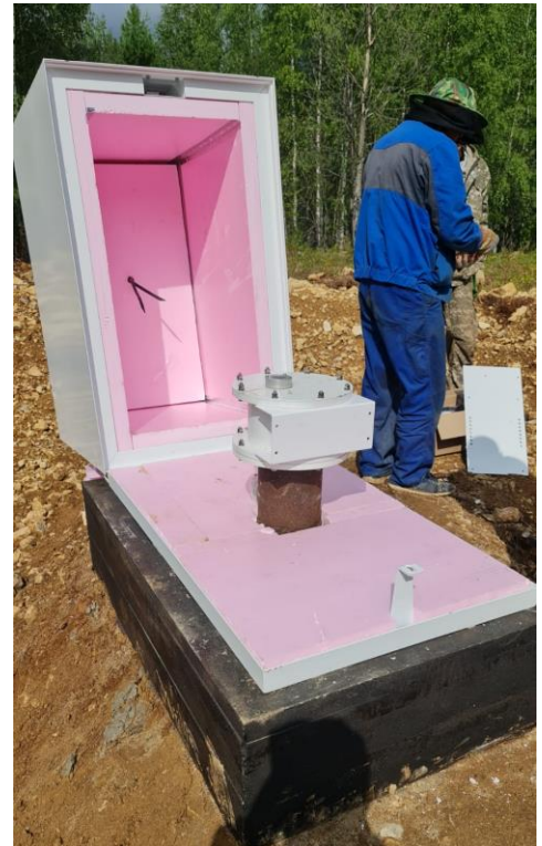
Figure 3. Example of a surface equipment vault, with digitizer and power and communication boxes.
