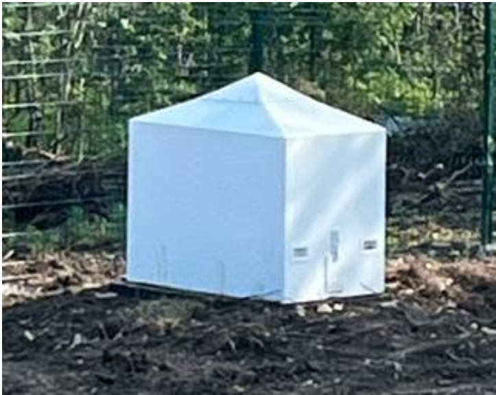
Figure 3. Example of a surface equipment vault, with digitizer and power and communication boxes.
