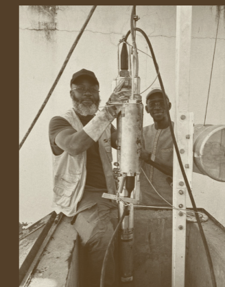
Outdated seismometer removed from borehole at auxiliary seismic station AS97, Babate, Senegal
